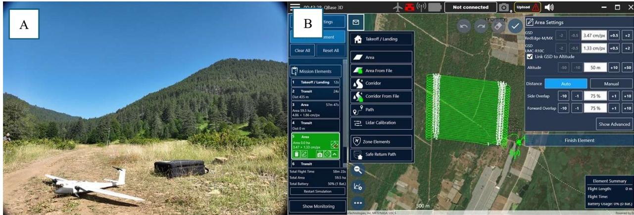
Figure 2. The Quantum Systems Trinity F90+ Fixed Wing VTOL UAV with the RGB Sony UMC R10C 20.1 MP camera payload (Left). Flight planning with QBase 3D software in Strofilia forest (Right).
