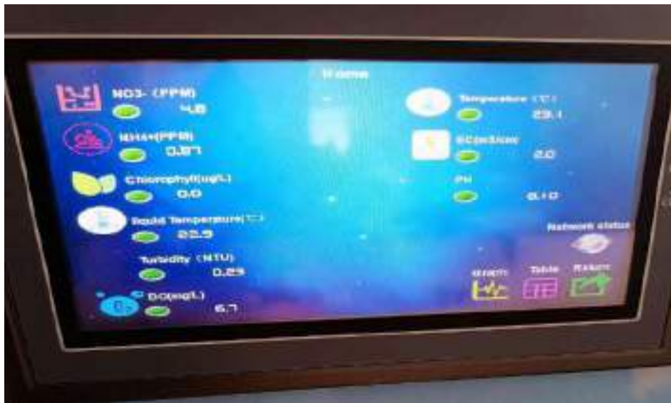
Figure 2. The touch screen interface of the RK900-1 terminal device.
